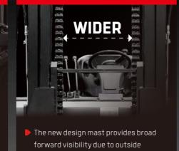
located hydraulic pipes of fork
